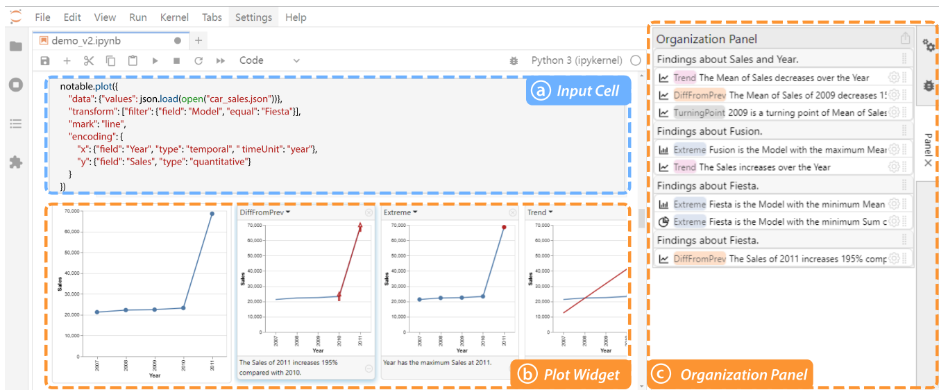
Figure 1: This figure illustrates the interface of Notable , an on-the-fly assistant for data storytelling in computational notebooks. (a) is an input cell where the chart is specified. The original chart and illustrated data facts are shown in (b), the plot widget . The plot widget allows users to modify and select useful data facts. The selected data facts are arranged into a story and displayed in (c), the organization panel . The automatically organized story can be further improved by users in the organization panel.
